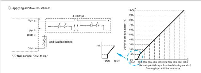
Note: 1. Min. duty cycle of output current is about 0.15%, and the dimming input is about  $6K\Omega$  or 0.6VDC, or 10V PWM signal with 6% duty cycle. 2. The duty cycle of output current could drop down to 0% when dimming input is less than  $6K\Omega$  or less than 0.6VDC, or 10V PWM signal with duty cycle less than 6%.
